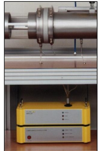
Fractional collection efficiency of oil mist separators, determined by means of a Topas Separator Performance Tester SPT 140
